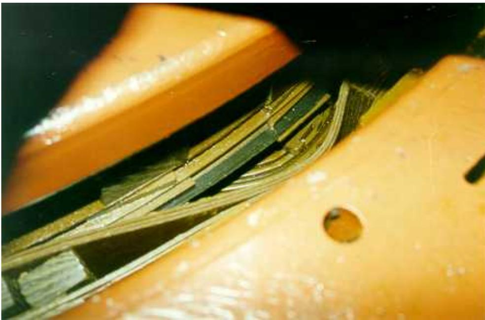
Top view on the common winding buckling in 200 MVA autotransformer
