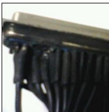
Fig 2: Conector DB 37 danificado
