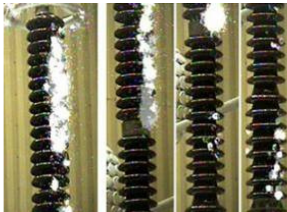
Figura A.6 – Coluna B2; 750 kV rms ; 5 mm/min
