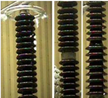
Figura A.4 – Coluna B2; 750 kV rms ; 1mm/min
