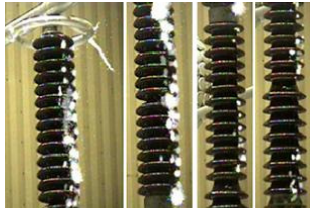
Figura A.5 – Coluna B2; 750 kV rms ; 3 mm/min
