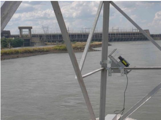
Figura 10. Trena Laser Instalada
