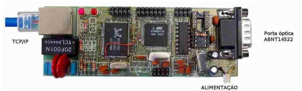
Figura 4 - Conversor ABNT14522 - TCP/IP (LACTEC – 2004)
