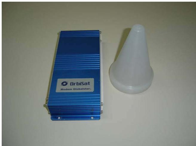
Fig. 2 – Antena e modem satelital.
