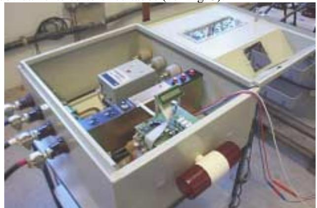
FIG. 3 – DETALHE INTERNO DO RELIGADOR
